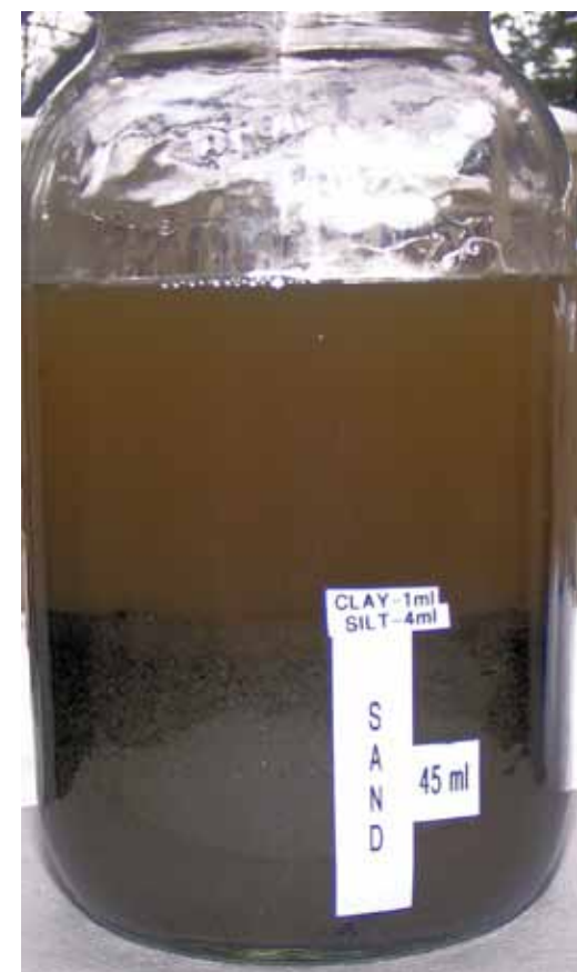
Figure 2. This soil texture test shows 90% sand, 8% silt and 2% clay. There is no dark organic layer. This soil will have problems holding water and plant nutrients. PHOTO: Leslie Welch.
