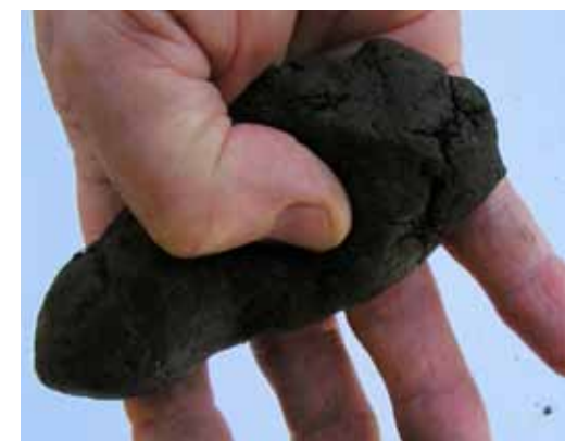
Figure 1. Clayey soils resist breaking down and stay in a ball. PHOTO: Leslie Welch.
